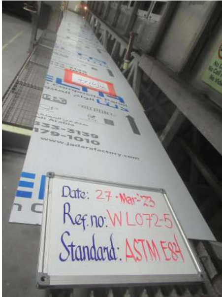
Photo 1: Specimen before the test. (Fire Side)
