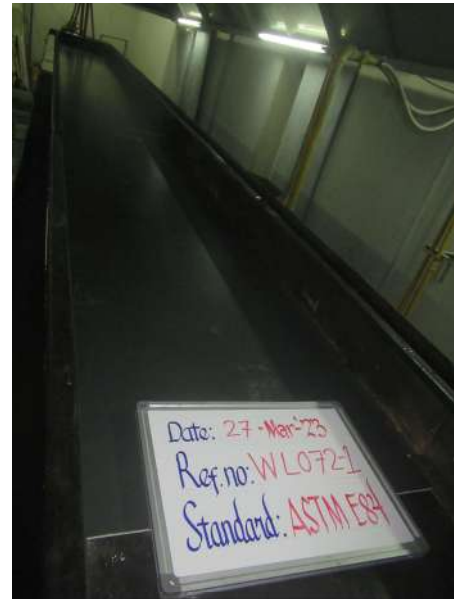
Photo 2: Specimen before the test. (Non-Fire Side)
