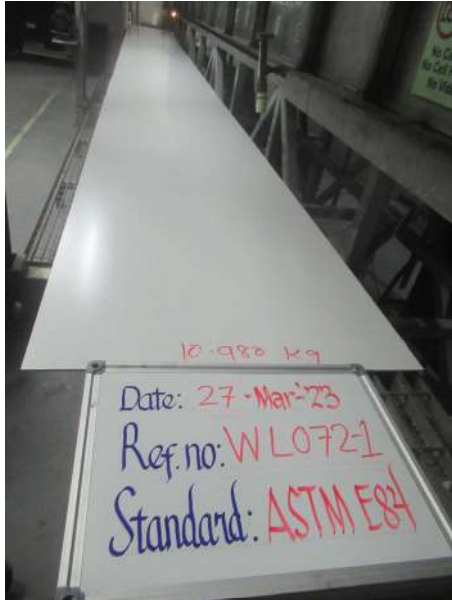
Photo 1: Specimen before the test. (Fire Side)
