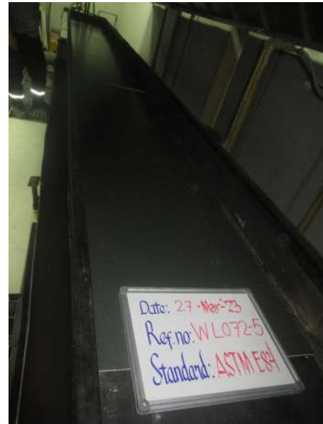
Photo 2: Specimen before the test. (Non-Fire Side)
